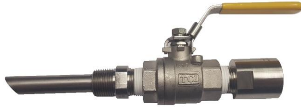
Depicted: QCC Series, 1/2" Injection Quill Assembly, 1/2" NPT, type 316 SS
